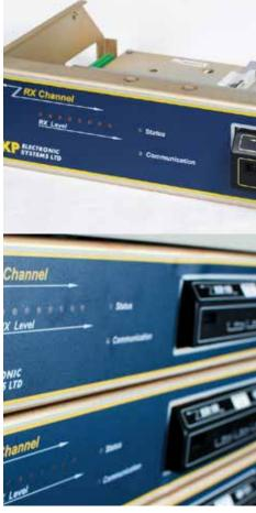
**OVERVIEW:** The MegaNet<sup>™</sup> Head-End is compromised of the RMR5000C and the MCM (Meter Control Management) software. The RMR5000C manages communication with RMR5000S Super Collectors, controlling collection processes and data flow ultimately feeding the MCM software.
